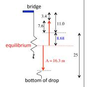
Minor note: The solid red line is where the axis would have to be put to effect this situation, and the dotted red line identifies where we are going 16.3 meters below equilibrium:
